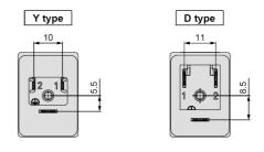
Circuit with indicator light (Built -in connector)
