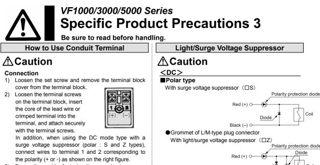
3) Secure the cord by fastening the ground nut.
