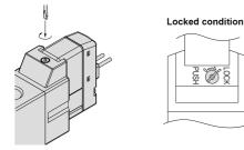
Push down on the manual override with a small flat head screwdriver until it stops. Turn it clockwise by 90° to lock it . Turn it counterclockwise to release it.
