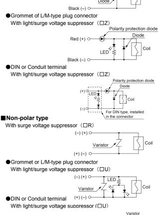
(-) (+) Coil (+) (-) Coil (+) (-) Coil For DIN type, installed in the connector
