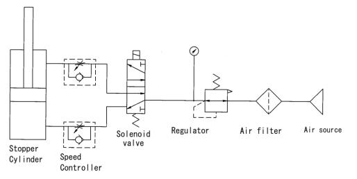
Fig. 8 Basic circuit of stopper cylinder (both double acting and double acting with spring)
