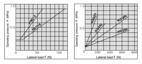
Fig. 2 Relation between Lateral load and operating pressure
