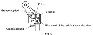
Please do not remove the grease applied to the piston rod end of the built-in shock absorber and periodically check the condition of the grease.
