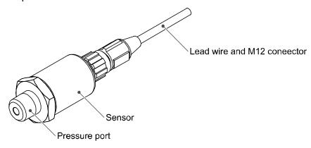
•Only fluids which are non-corrosive to C3604 + electroless nickel plated, Al203 (aluminum oxide) and FKM should be used.
