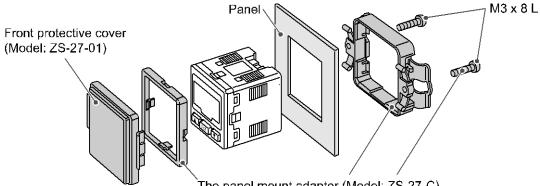
The panel mount adapter (Model: ZS-27-C) can be rotated by 90 degrees for mounting.
