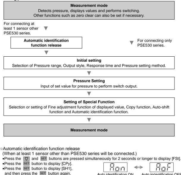
•If [Aon] is displayed, press the ( or ) button (Only PSE530 series) to display [AoF], and then press the **SET** button.
