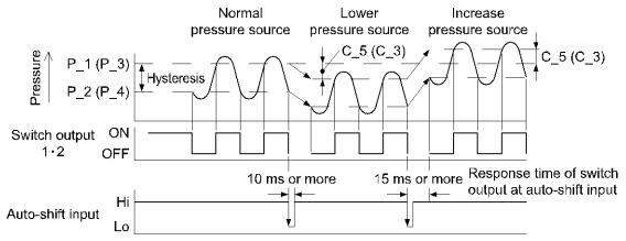
•Using with auto-shift input, accepted setting range is like below
