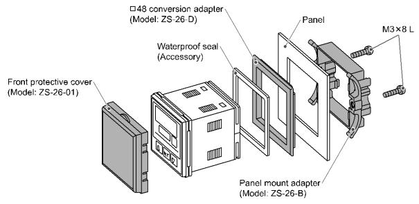
\*: The panel mount adapter can be rotated by 90 degrees for mounting.
