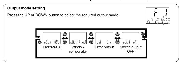
Press the SET button to set. Move on to reversed output setting.
