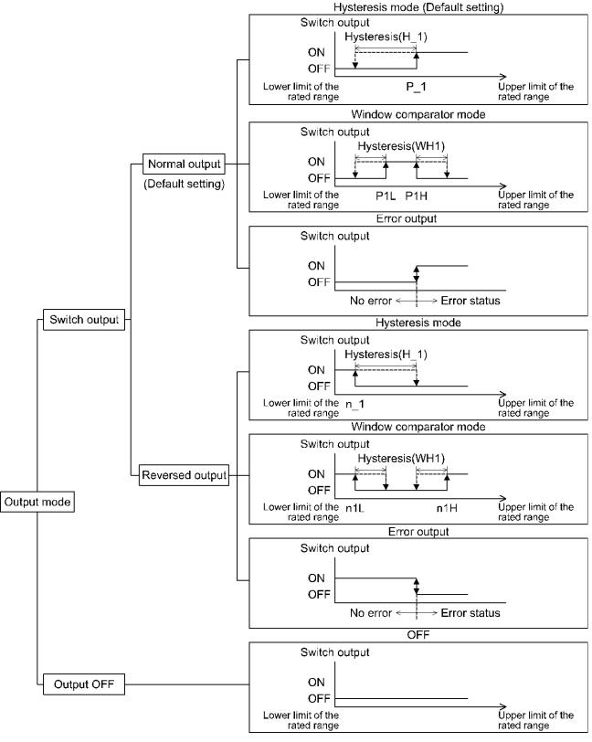
If the point at which the switch output changes is outside of the set pressure range due to the selection of normal or reversed output, the hysteresis value is automatically adjusted.
