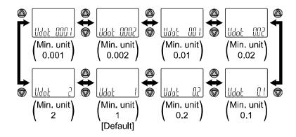
Move on to the setting of the lower limit of the additional rated range.
