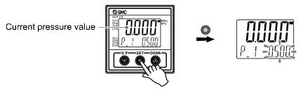
(2) Press the UP or DOWN button to change the set value. The set value can be increased with UP button and can be reduced with DOWN button.
