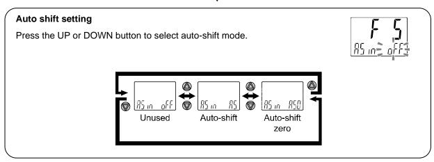
Press the SET button to set. Move on to setting of effective output.
