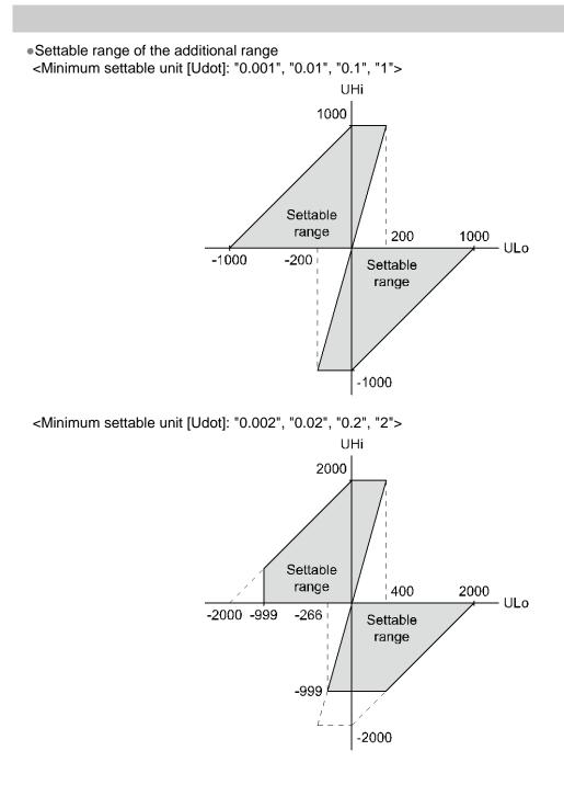
\*: When flow range, minimum unit/lower limit/upper limit of additional range is changed, setting below will be initialized and cleared. These items must be set again.
