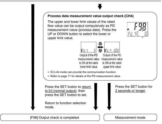
\*: Measurement mode can return from any setting item by pressing the SET button for <u>2 seconds or longer</u>.
