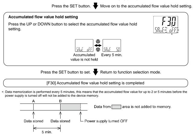
When the power supply is turned on again, the accumulated flow count will start from the value recorded at B.
