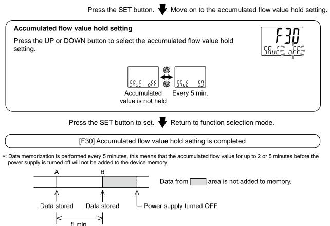
When the power supply is turned on again, the accumulated flow count will start from the value recorded at B.
