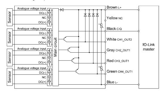
•When used as a switch output device Load current 80 mA Internal voltage drop: 1.5 V or less
