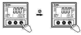
•When the UP and DOWN buttons are pressed and held simultaneously for <u>1 second or longer</u>, the set value is displayed as [- - -], and the set value will be the same as the current flow value automatically (snap shot function (Refer to page 66)). Afterwards, it is possible to adjust the value by pressing the UP or DOWN button.
