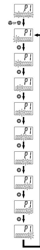
When the SET button is pressed for <u>1 second or longer</u>, [000000000] will start flashing.
