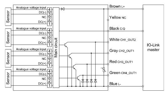
•When used as a switch output device Max. applied voltage: 30 V, Load current 80 mA Internal voltage drop: 1.5 V or less
