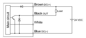
Maximum applied voltage: 28 V Maximum load current: 60 mA Internal voltage drop 1.5 V max.
