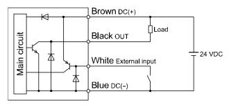
Maximum applied voltage: 28 V Maximum load current: 60 mA Internal voltage drop 1.5 V max.
