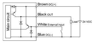
Maximum load current: 60 mA Internal voltage drop 2 V max.
