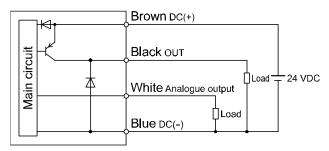
Maximum load current: 60 mA Internal voltage drop 1.5 V max.
