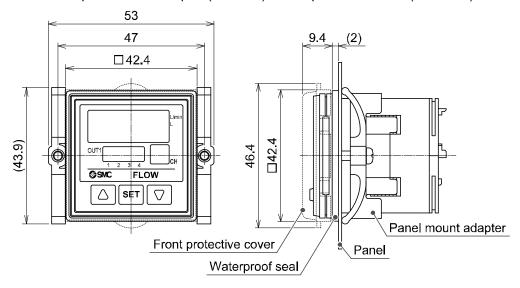
PF2#20# + panel mount adapter (ZS-26-B) + front protective cover (ZS-26-01) + □48 mm conversion adapter (ZS-26-D)
