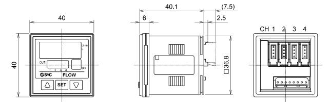
PF2#20# + panel mount adapter (ZS-26-B) + front protective cover (ZS-26-01)
