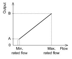
\*: Analogue output is based on the rated flow range at normal condition.
