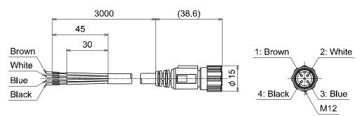
Lead wire and connector (Right angle): ZS-37-B
