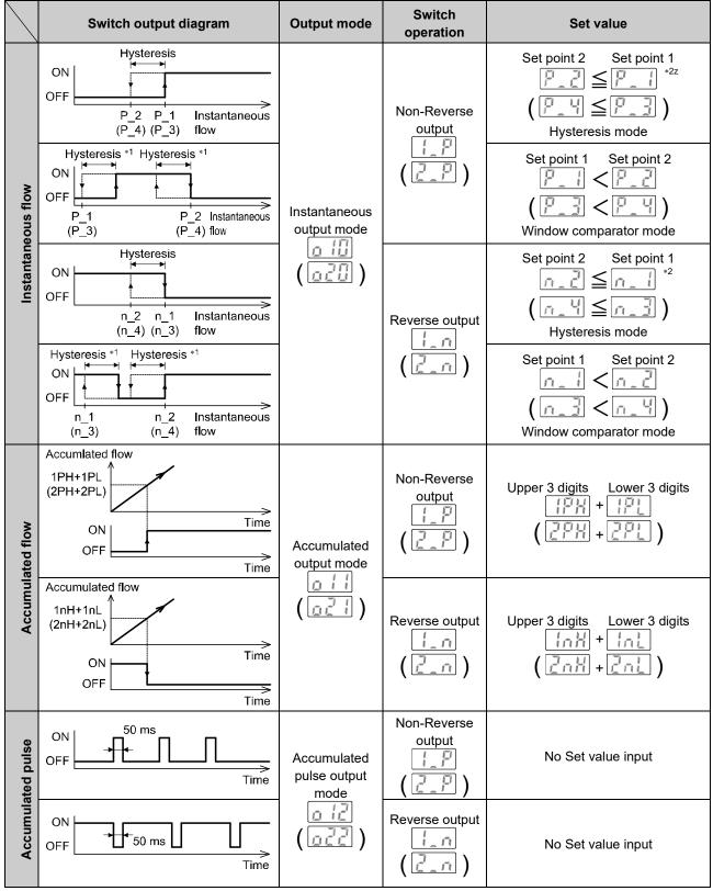
\*1: In window comparator mode, the hysteresis is fixed at 3 digits. When setting, allow 7 digits or more between Set point 1 and Set point 2 (Set point 3 and Set point 4).
