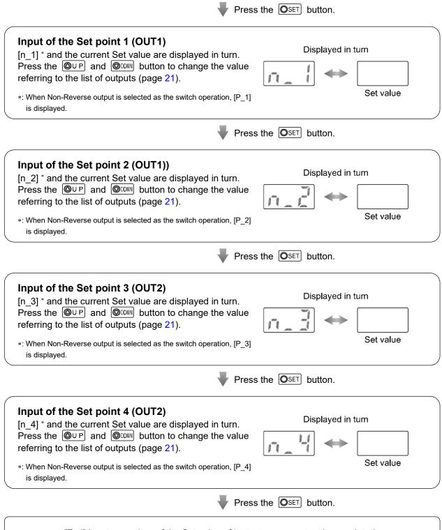
[F\_1] Input procedure of the Set value of instantaneous output is completed. Return to measurement mode.
