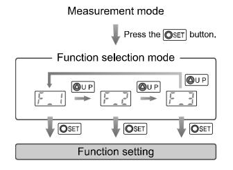
\*: When OUT1 or OUT2 is assigned to be instantaneous output mode during initialize mode, [F\_1] and [F\_2] are displayed. When OUT1 or OUT2 is assigned to be accumulated output mode, [F\_3] is displayed.
