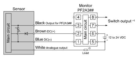
Analogue output: 4 to 20 mA Load impedance: 300  $\Omega$  (12 VDC) 600  $\Omega$  (24 VDC)
