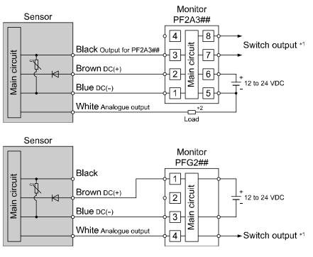
Analogue output: 1 to 5 V Output impedance: 1  $k\Omega$
