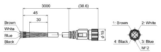
Lead wire and connector (Angle): ZS-37-B
