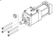
6) Confirm that the operation of 5) is performed correctly, and then tighten the lock unit holding bolt with an appropriate tightening torque as shown in the table below.
