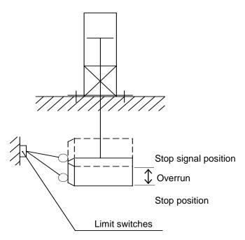
Fig. 5 Overrun of intermediate stop
