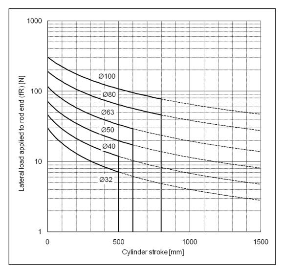
Chart 9 Allowable lateral load applied to rod end
