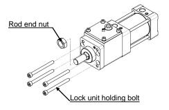
3) Pull out the old lock unit from the cylinder.
