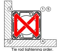
Appropriate tightening torque for tie-rod nuts
