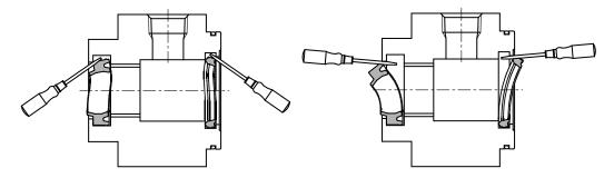
Fig. 16 Removal of rod seal and cushion seal
