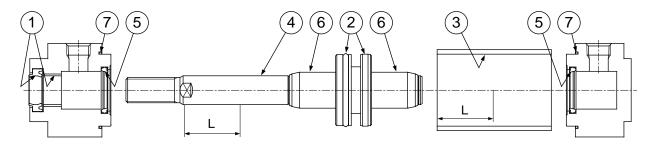
Fig. 18 Position for application of grease
