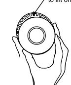
Fig 17 How to remove piston seal
