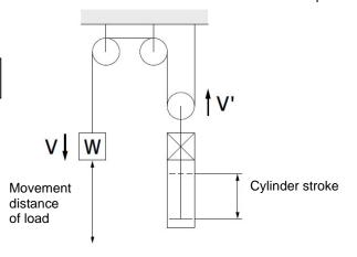
Fig. 1 Double speed mechanism
