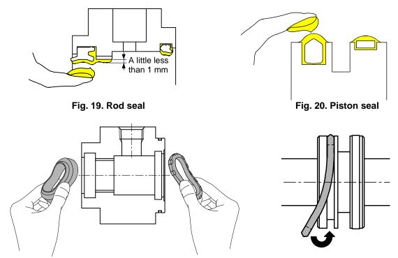
Fig. 21 Mounting of the rod seal and cushion seal
