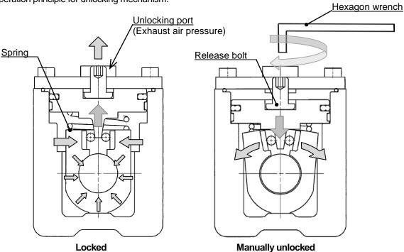
Fig.6 Operation principle of locking mechanism
