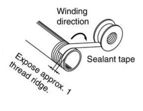
Fig. 4 Sealant tape
