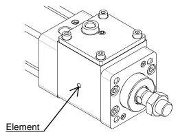
Fig. 3 Lock unit element
