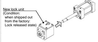
5) Insert the lock unit holding bolt and tighten it temporarily. Check that the piston rod operates smoothly by hand while maintaining the lock release state.
