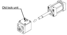
4) Insert a new lock unit into the cylinder. The lock unit for maintenance is supplied with lock released state at the shipment from the factory.
