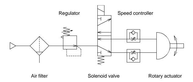
Fig.1 Basic circuit
