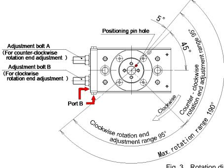
Fig. 3 Rotation direction and rotation angle
