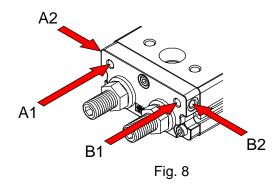
Rotary table ports have a fixed orifice. Do not make the diameter of this hole larger by additional processing.
