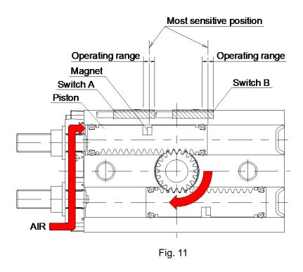
When switch A is turned on and pressure is supplied in the direction indicated by the arrows in Fig. 11, the piston moves and the table rotates clockwise.
