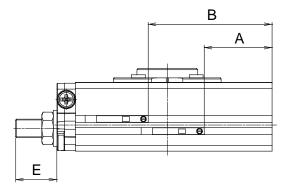
Table 15. Dimension E [mm] Adjust-Shock Size ment bolt absorber 10 17 31 20 25 35 30 23 50 33 53
