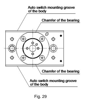
(5) Mount the end cover assembly on the body.
