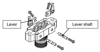
(5) Pull out the rod cover and piston assembly and replace the seal.
