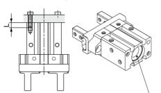
Use the holes on the body end surface for positioning.
