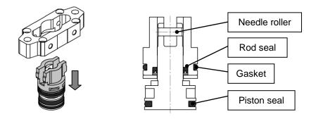
Assembly should be performed by following the removal procedure in reverse. Refer to the disassembly drawing for the tightening torque for the bolt. Use a specified grease. Specified grease pack part number: GR-S-010(10g)
