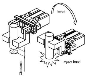
3. <u>Adjust the gripping point so that an excessive force will not be applied to the fingers when inserting a workpiece.</u>
