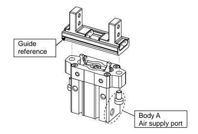
(2) The guide may be displaced during tightening of the guide bolts. In order to avoid this displacement, place the guide and Body A on a flat surface and insert a spacer to fill the gap between the surface and guide (with reference line face down).
