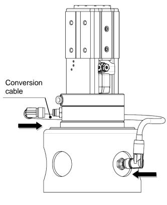
How to Mount Magnet Gripper (MHM-25D-X7400A-HC10DT,HC10)
