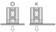
• If multiple magnet grippers are used for transferring a workpiece with a large surface area, properly allocate the magnet grippers to maintain balance.
