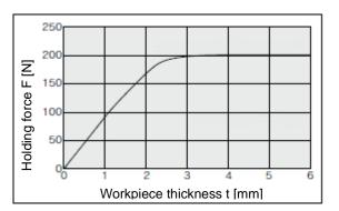
The holding force graph shows the theoretical value for low carbon steel plate. Holding forces very depending on the material and shape of the workpiece. Please perform a holding test referring to the value selected based on the graph.
