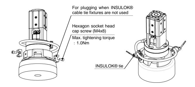
$^{\star}$  Use a cross recessed resin round head screw (M4 x 6) as a plug when the INSULOK® cable tie is not used.
