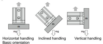
•Thin workpieces may be deformed during transportation. It is recommended to use multiple magnet grippers for scenarios such as this.
