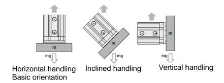
Thin workpieces may be deformed during transportation. It is recommended to use multiple magnet grippers for scenarios such as this.
