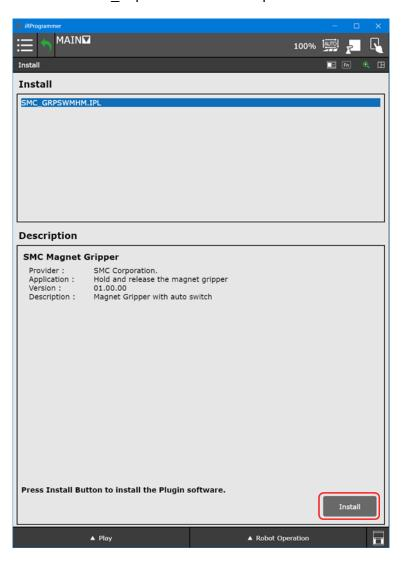
4. Tap "OK" and install the "SMC Magnet Gripper" Plugin software.
