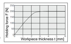
The holding force graph shows the theoretical value for low carbon steel plate. Holding forces very depending on the material and shape of the workpiece. Please perform a holding test referring to the value selected based on the graph.
