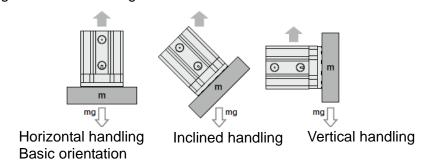
Thin workpieces may be deformed during transportation. It is recommended to use multiple magnet grippers for scenarios such as this. Calculate the required holding force.
