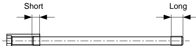
Fig. 11 Tie Rod Threading Directionality
