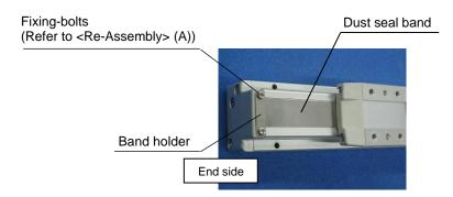
2. Remove the "Seal band holder" and the "plate" as shown.
