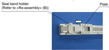
3. Loosen the fixing bolts of motor side of the "Band holder" and then remove the "Dust seal band".
