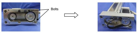
4. After "Belt" is installed, and the bearing support is obtained, the root of "Motor" is pulled in a string or a long banding band. With tensile force adjusted, tighten the bolts which fix the actuator to the motor. (See the table below)
