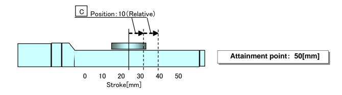
Condition 2) 30mm position  $\rightarrow$  **Step no.1**  $\rightarrow$  **Step no.1** (Move Method: Relative)
