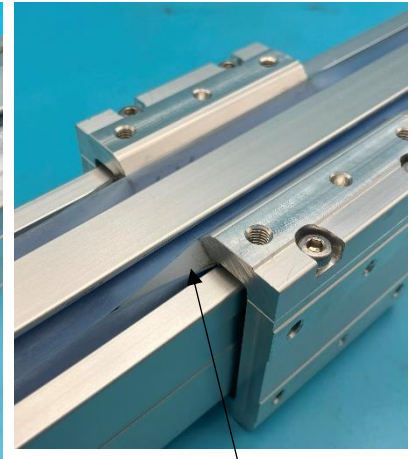
Abnormal (Grease is lost)
