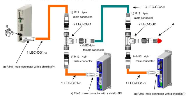
Description No Part number Content 1 Communication cable cable LEC-CG1-Cable to connect the gateway unit CN1 and the branch 0.3m connector, or controller (LEC) CN4 and the branch connector. 0.5m 1 1m LEC-CGD Branch connector The junction cable to connect the gateway and the controller. Cable between branches LEC-CG2-□ Cable to connect the branch connector. K 0.3m 0.5m 1 1m Terminating Resistor Termination on RS-485 Bus (120 Ohms) Recommended connector :XS2C-D4\*\* [OMRON Corporation]
