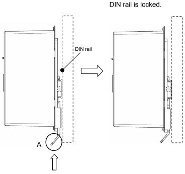
Hook the controller on the DIN rail and press the lever of section A in the arrow direction to lock it.
