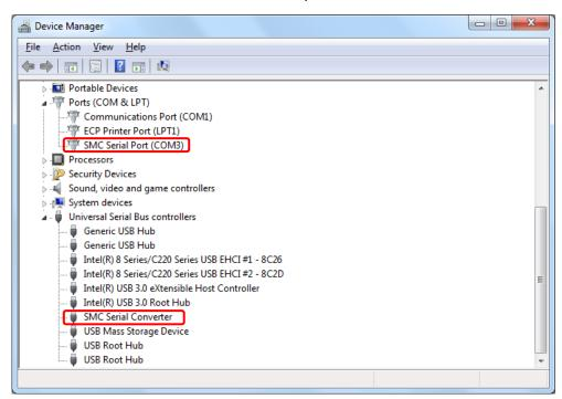
The communication port number is needed when starting this software.
