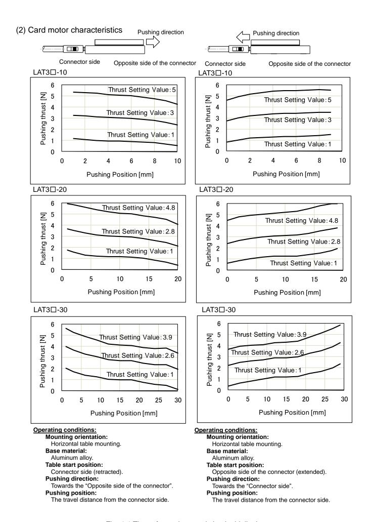
Fig. 4-1 Thrust force characteristics (guideline).
