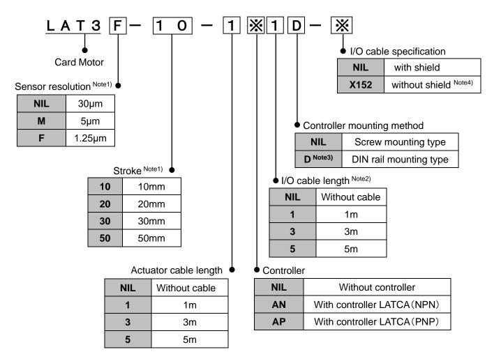
Note1) Refer to the table below for the Card motor model resolution and stroke available.
