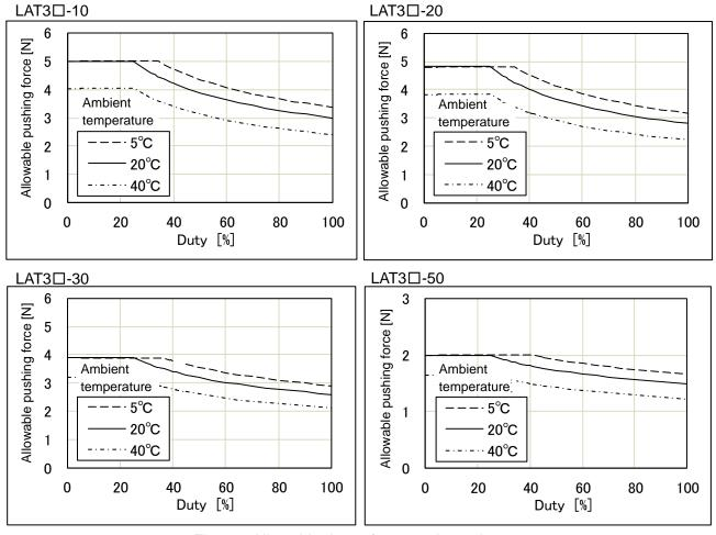
Fig. 4-3 Allowable thrust force setting values.
