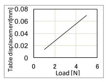
Fig4-5 Table displacement (guideline)
