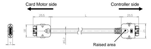
Note) The actuator cable is direction dependent.
