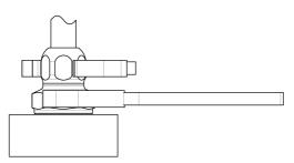
(5) Fix the body with a tightening tool. Tighten the union nut to the end surface of the body using a suitable wrench.
