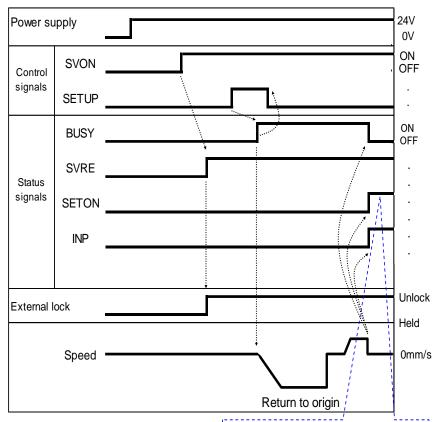
INP signal is ON when the current position is within the step data position range. Otherwise, the signal is OFF
