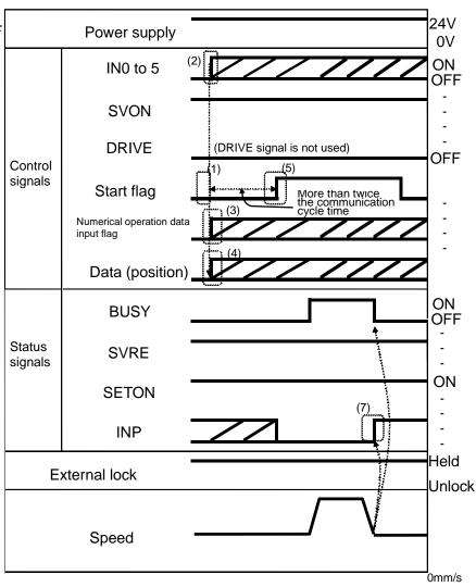
(5) Input the numerical operation data input flag bit and numerical operation data, and then, input 7012h, bit0: Start flag=ON.
