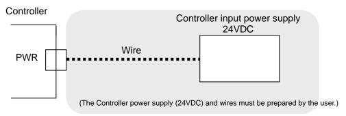
\* Refer to 6. Details of Power supply plug (P.22) for wiring.
