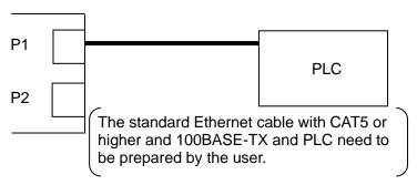
\* Cable can be connected to either P1 or P2.
