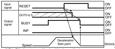
\* INP is ON when stop position is within the positioning range.
