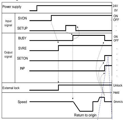
INP signal is ON when the current position is within the step data position range.
