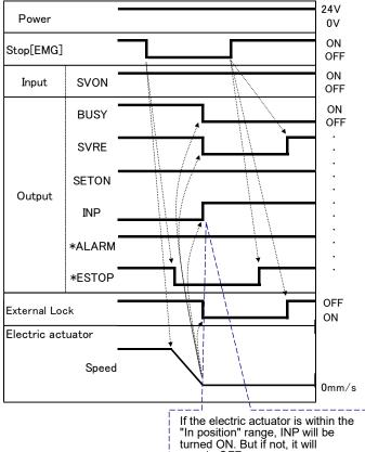
The "\*ALARM" and "\*ESTOP" are expressed as negative-logic circuit. When "Stop" is OFF, the stop is activated.
