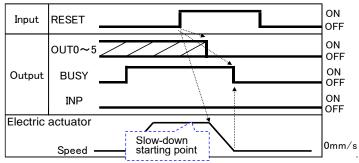
If the electric actuator is within the "In position" range, INP will be turned ON.
