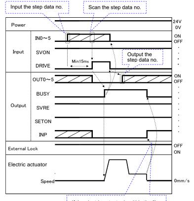
If the electric actuator is within the "In position" range, INP will be turned ON but if not, it will remain OFF.
