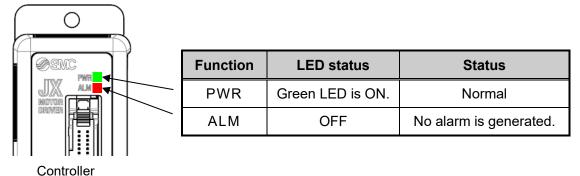
If the LED [PWR] lights in green, the controller is in the normal condition.
