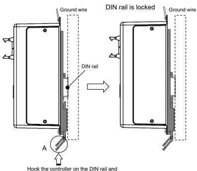
Hook the controller on the DIN rail and press the lever of section A in the arrow direction to lock it.
