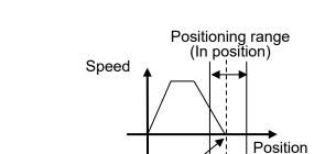
Positioning operation [Speed/ Position] (Example)
