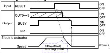
If the electric actuator is within the "In position" range, INP will be turned
