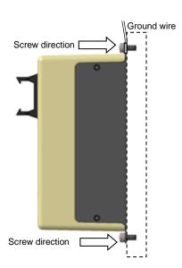
(Installation with the DIN rail)
