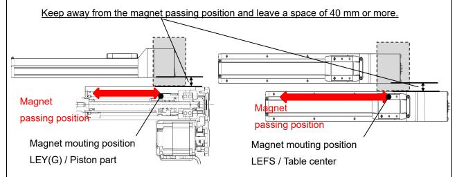
The motors of the electric actuator can be installed close to each other.
