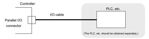
Please refer to "6.4 Parallel I/O Wiring Example" for how to wire the Parallel I/O connector.
