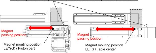
The motors of the electric actuator can be installed close to each other.
