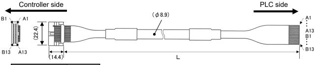
Number of Ways 26 AWG AWG28 The separate lines of the terminal on the PLC side are twisted together with an adhesive tape with a pitch of 2.54 mm.
