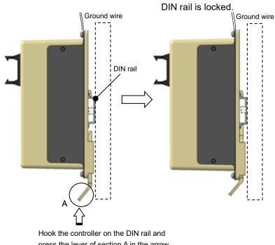
press the lever of section A in the arrow direction to lock it.
