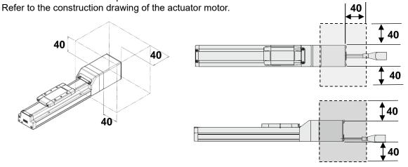
Air cylinder installation with an auto switch is forbidden in the shaded area.
