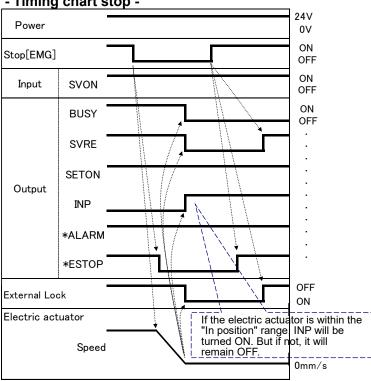
The "\*ALARM" and "\*ESTOP" are expressed as negative-logic circuit. When "Stop" is OFF, the stop is activated.
