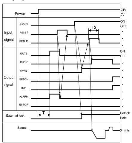
T1: 1.6 s or less (System initialize time + Time required to activate alarm)
