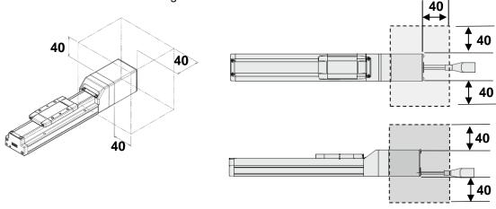
Air cylinder installation with an auto switch is forbidden in the shaded area.
