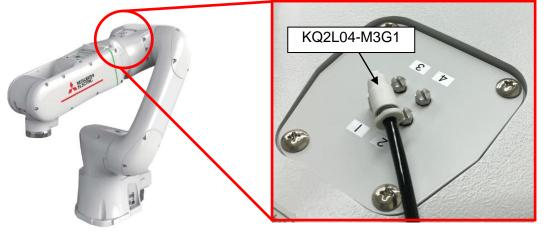
2) Connect the One-touch fitting and air gripper with a coil tube (TCU0425B-1).
