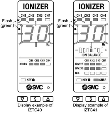
Example of frequency setting mode for CH1.
