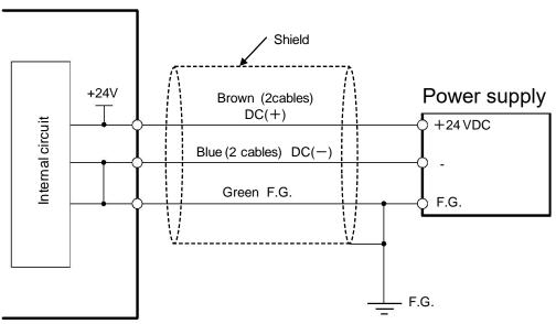
Make sure to ground the F.G. cable (green) with a resistance of 100 ohms or less. Without grounding, this products and/or power supply may be damage.
