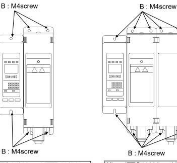
When IZTC41(-L) and IZTP41(-L) are directly connected.
