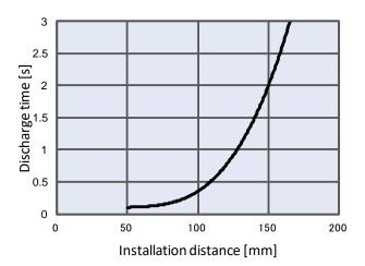
2) With High speed static neutralization cartridge With air purge, For IZT42-112D
