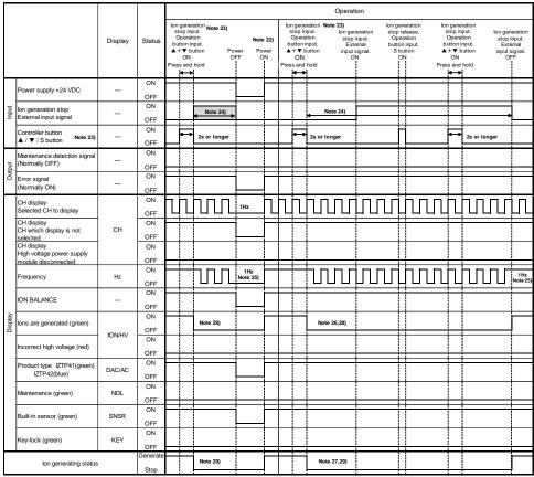
Note 22) It takes 3 seconds to operate after the power is on.
