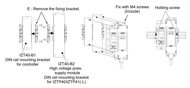
II. When the controller and high voltage power supply module are connected by separate cable
