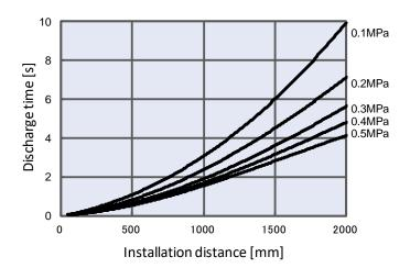
3) With Energy saving static neutralization cartridge With air purge, For IZT42-112L
