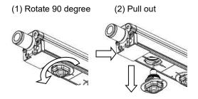
Removal procedure of emitter cartridge
