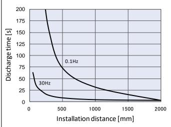
With Energy saving high-efficiency cartridge For IZT42-112V
