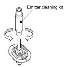
d. When the emitter cartridges are removed for cleaning, remount them to the bar according to the "Mounting procedure of emitter cartridge" shown below. Make sure that the cartridges are securely mounted. If not, the cartridges may become dislodged when compressed air is supplied to the ionizer.
