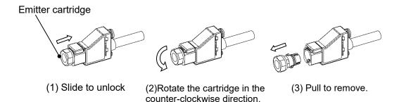
Removal procedure of the emitter cartridge
