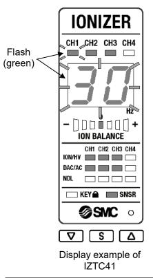
Example of frequency setting mode for CH1.
