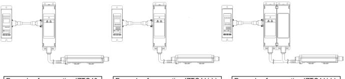
Example of connecting IZTC40, IZTP40 and IZTB40 (IZT40) Example of connecting IZTC41(-L), IZTP41(-L) andIZTB40 (IZT41(-L)) Example of connecting IZTC41(-L), IZTP42(-L) and IZTB42 (IZT42(-L))
