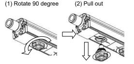
Removal procedure of emitter cartridge
