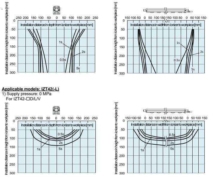
With High speed static neutralization cartridge, Supply pressure: 0.3 MPa For IZT42-□D
