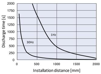
With Energy saving static neutralization cartridge For IZT40-112L, IZT41-112L
