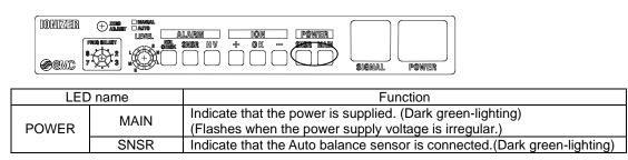
• ION LED: Indicates the polarity of the discharge ion and the offset voltage status.
