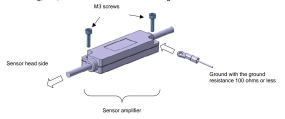
Recommended crimped terminal: TMEN1.25-3, an insulation coated crimped terminalmanufactured by Nichifu. Co.Ltd.
