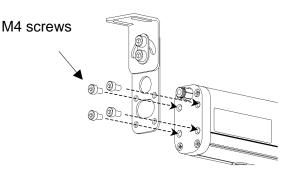
(3) Mount an intermediate bracket onto the center of the ionizer body.
