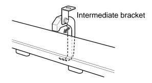
(4) Tap M5 screw threads for the mounting brackets in the location the ionizer is to be installed. Attach the ionizer body and brackets with M5 screws.
