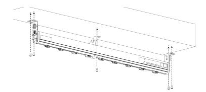
(5) Adjust the angle of the ionizer body to make the static neutralization effective, and fix with the rotating set screws (M5) of each bracket.
