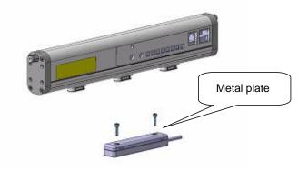
(2) Installation of sensor amplifier
