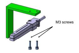
Due to the construction of the sensor, the sensor head housing is shared with GND. Install and supply power with great caution to avoid short-circuit with the +24 V power supply.
