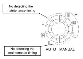
H (High) Level that does not affect the static neutralization time. M (Middle): Level at which the static neutralization time is a little bit
