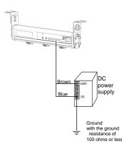
\* Make sure to ground DC1(-) lead wire [Blue] of the power supply cable with the ground resistance of 100 ohms or less. Otherwise, breakage may occur.
