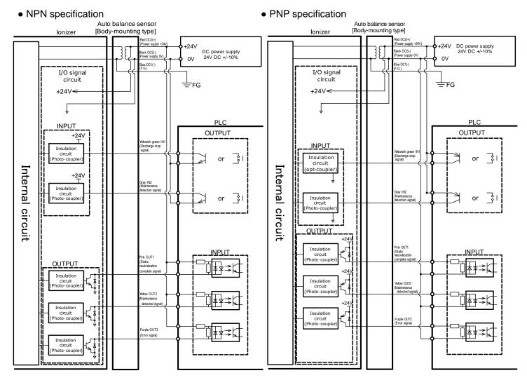
\* Make sure to ground the DC(-)[Blue] with the ground resistance of 100 ohms or less directly. Not necessary to connect the power supply GND. If connecting with GND, All I/O signal lines are not isolated from FG.
