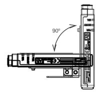
Mounting angle adjustable range of the pivoting bracket
