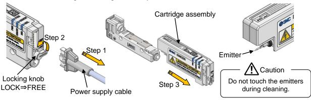
4. Clean the emitter mounted to the cartridge assembly.
