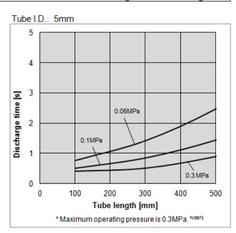
Note 1) Refer to "Cautions when using the IZN10E-11□□□-□ (Female threads for piping)" on page 9.
