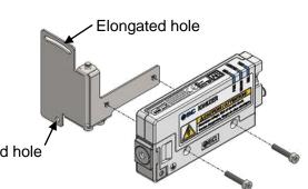
b. Fixing of the bracket
