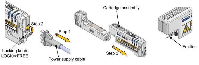
The procedure for mounting the cartridge assembly is the reverse of removal. Confirm that the Locking knob is in the FREE position.
