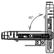
Mounting angle adjustable range of the pivoting bracket
