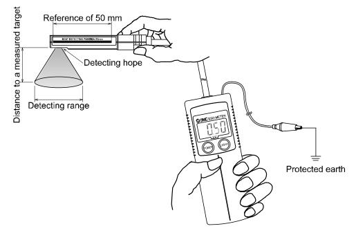
\*: The detecting range of the sensor is 180 mm (at the best measurement distance of 50 mm).
