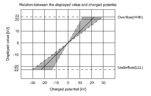
There will be difference between the actual value and displayed value of charged potential depending on the measuring distance between the measured target and the sensor. The shaded part shows the deviation in a measuring distance range of 25 to 75 mm.
