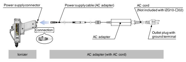
Note) The rated voltage of the AC cord supplied with IZG10-□01 is 125V, and the plug is JIS C8303 type B, which is for Japanese domestic use. If the product is used in an area other than rated voltage (220 or 240VAC), select IZG10-□02 without AC power cord and prepare an AC cord with ground terminal inlet IEC60320-C13 adapted to the power supply voltage.
