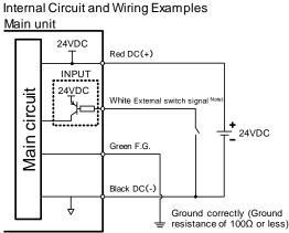
Note) The external switch signal consists of a trigger input and an OR circuit. When the external switch signal is not used, cut the semi-strip processing section to prevent the conductor from making contact.
