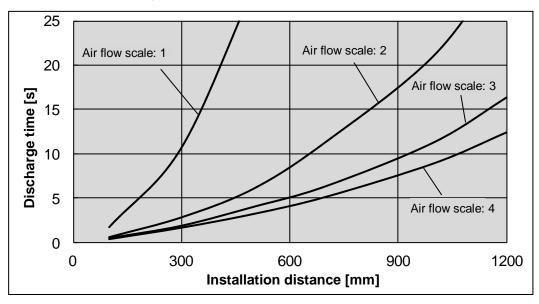
2) Discharge characteristics range (Discharge time from 1000 V to 100 V)
