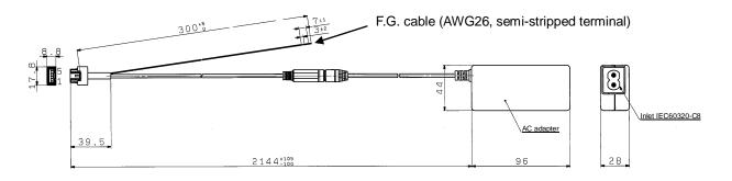
Note) The AC cord is only for use in Japan. (Rated voltage 125 V, Plug JIS C8303, Inlet IEC60320-C8) External output cannot be used when the AC adapter is being used.
