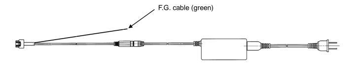
Note) The AC cord is only for use in Japan. (Rated voltage 125 V, plug JIS C8303, Inlet IEC60320-C8) External output cannot be used when the AC adapter is being used.
