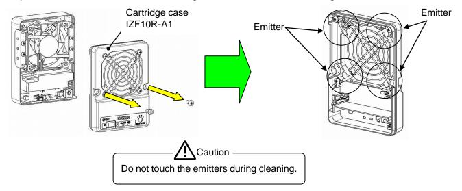
3) Four emitters are fixed in the cartridge case enclosure, so clean the end of each of the emitters. Make sure that all four emitters are cleaned.
