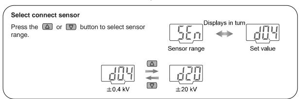
After selecting sensor range, press the  $\triangle$  and  $\nabla$  button together.
