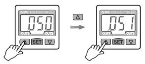
•Press the button once to decrease by one figure and press it continuously to keep set figure decreased.
