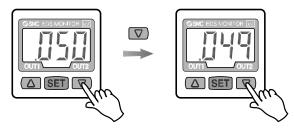
4. Press the **SET** button to finish the setting. Then [P\_2] is displayed. **Set** as above.
