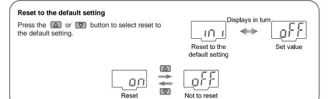
Press the **SET** and **V** buttons simultaneously for 5 s. or more when "ON" is displayed.
