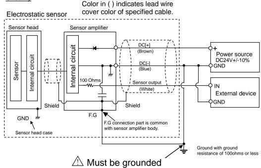
GND shall be grounded to earthing resistance of 100 ohms or less. Exclusive power supply is recommended for the power to actuate the sensor. If other components are connected to this power supply when static electricity is discharged to the sensor head or noise interrupt GND, connected component could malfunction or be damaged.
