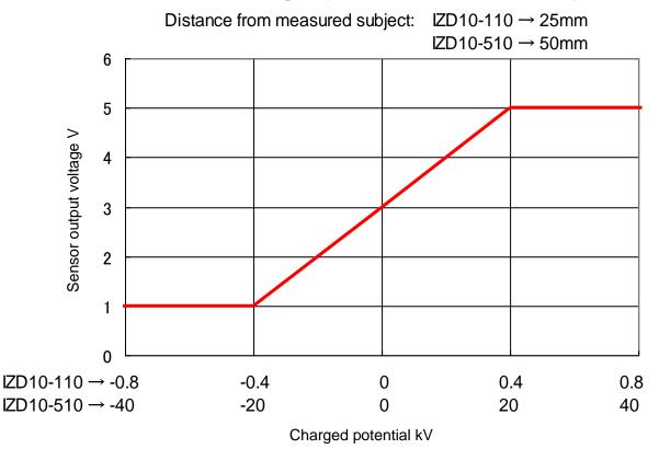
Relation between the output voltage of the electrostatic sensor and detected charged electricity depends on the distance between the sensor head and measured object. (See "6-1 Output signal" for the relation between the output voltage of the electrostatic sensor and detected charged potential based on installed distance )
