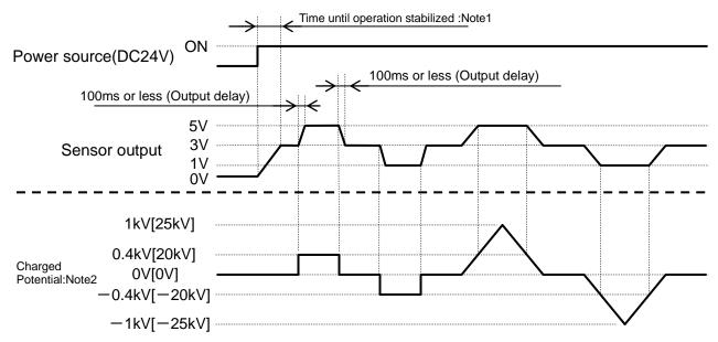
Note1: Although the sensor becomes operable one second after supplying the power, values may be unstable. It is recommended to wait for 10min. or longer for start operation.
