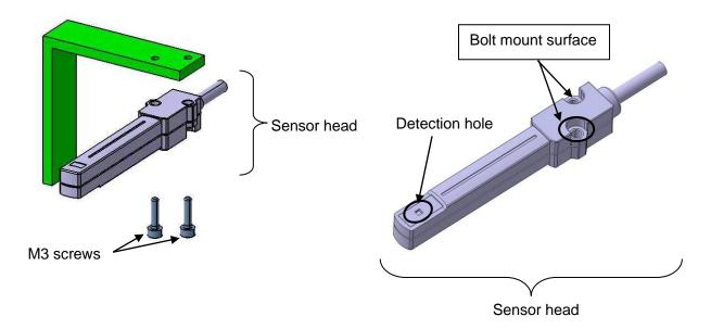
Mate M3 bolt to the bolt mount surface. Mounting from the opposite side leads to cause the breakage of the sensor head.
