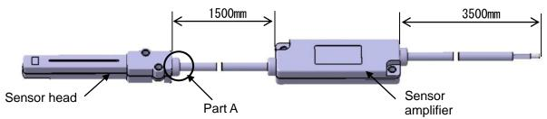
Electrostatic sensor has two types of sensors below.
