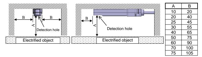
(2) After installation, confirm if electrified potential is correctly measured.
