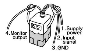
The optional cable connector is a 4 wire type. When the monitor output (analogue output or switch output) is not being used, prevent the unused wires from touching the other wires, as a malfunction could occur.
