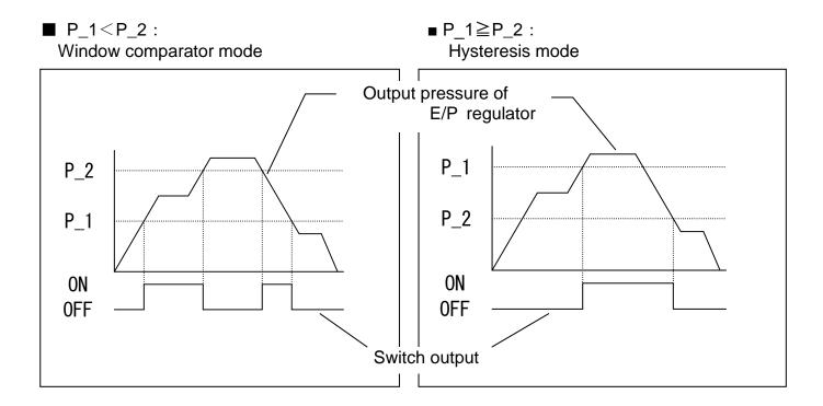
■ P\_1=P\_2=0 : Out of range mode (The switch output turns on when set pressure is achieved.)
