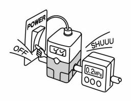
If the power supply to this product is turned off due to a power failure during normal operation, the output on the secondary side will be held and air will flow continuously.
