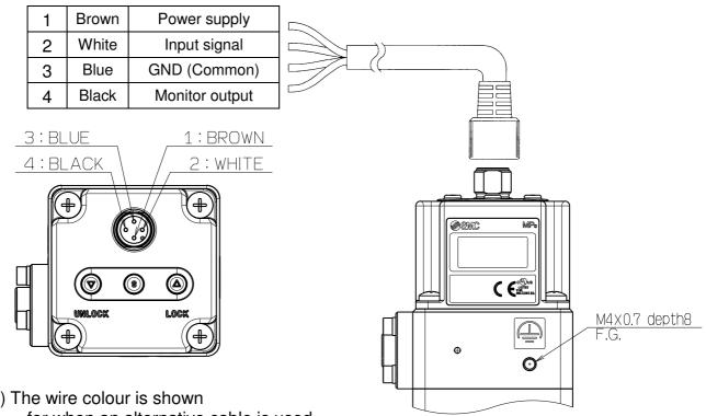
(Note) The wire colour is shown for when an alternative cable is used.
