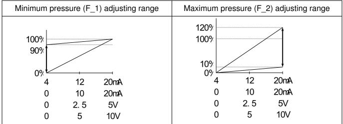
(Note1) F\_1 is adjustable in a range from 0% to 90% of the rated value.
