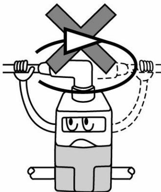
Please note that the right angled cable connector does not rotate and is limited to only one entry direction.
