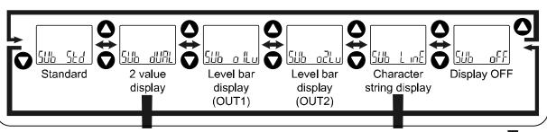
[dUAL] 2 value display is selected. Press the SET button to move on to sub display (left) setting.
