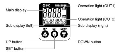
Operation light: Displays the switch operating condition.
