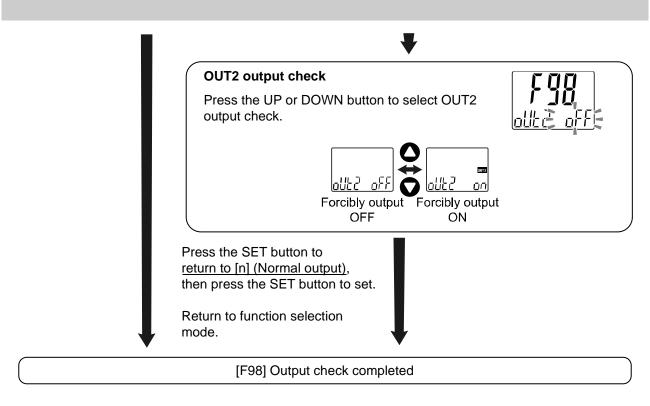
\*: Measurement mode can return from any setting item by pressing the SET button for 2 seconds or longer.
