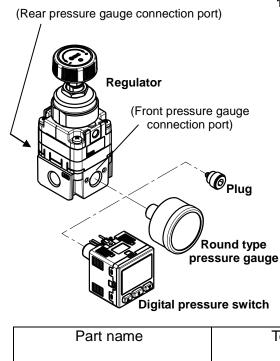
1) Instruction for mounting of the round type pressure gauge and digital pressure switch
