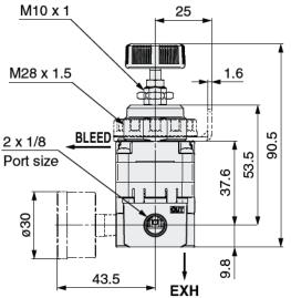
With digital pressure switch: IR10□0-01□E□-A
