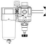
③ Non-flexible piping materials such as steel piping will be subject to excessive moment load and vibration from the piping side, so use a flexible tube for intermediate connections.
