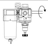
② Do not apply any additional twisting, or bending moments except for the weight of the filter regulator itself.
