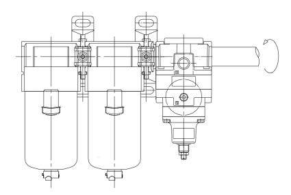
(2) Do not apply torsion or bending moment other than the weight of the product itself. The external piping should be supported separately because it may cause breakage.
