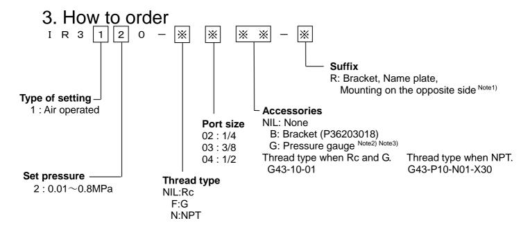
(Note 1) In the standard mounting position, the product name plate is attached to the front and the bracket is mounted to the back when viewed with the SUP side on the left and OUT side on the right.
