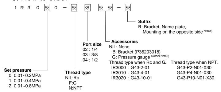
(Note 1) In the standard mounting position, the product name plate is attached to the front and the bracket is mounted to the back when viewed with the SUP side on the left and OUT side on the right.
