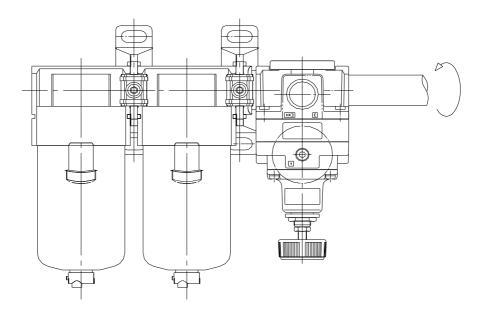
(2) Do not apply torsion or bending moment other than the weight of the product itself. The external piping should be supported separately because it may cause breakage.
