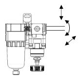
③ Piping materials without flexibility such as steel tube piping are prone to be effected by excess moment load and vibration from the piping side. Use flexible tubing in between to avoid such an effect.
